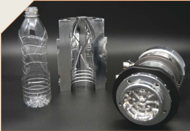
Whether made out of glass, PET or aluminum, Krones Inc. machines and processes millions of bottles, cans and specially-shaped bottles each day, including this mold for a plastic bottle.
