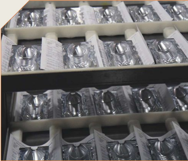
Krones makes very tight-tolerance, similar mold parts at each one of its locations, all requiring high accuracy and highly-polished surface finishes down to Ra right out of the five-axis machine.
